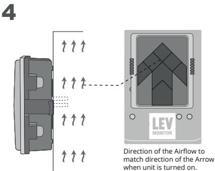
Place the LEV Monitor spigots into the duct with the Arrow pointing in the direction of the Airflow.
