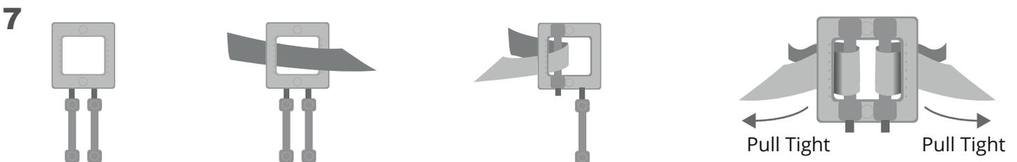
Feed the strap ends through the bracket as shown and pull tight to secure on either side of the unit then back around until both ends meet.
