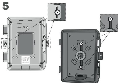
**Fastening Option 1:** The LEV Monitor can be secured to larger ducts using external flanges.
