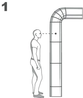
Select a suitable mounting position ensuring the LEV Monitor is clearly visible, unobstructed and downstream of any dampers.
