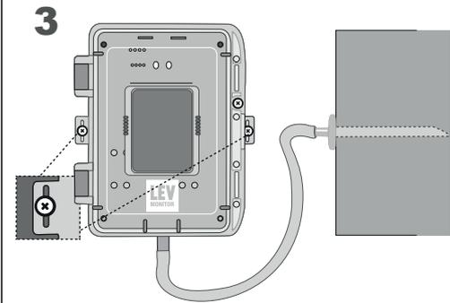
For wall fixing, mount the LEV Monitor in a visible location, insert and screw the spigot into the duct, then connect the monitor and probe using the hose provided.
