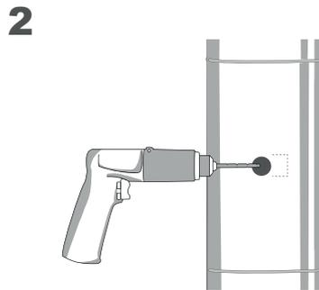
Drill a 8mm hole in to the duct and ensure that all edges are de-burred to avoid tearing the seals.
